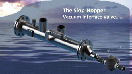
The Slop-Hopper is a large scale vacuum interface valve which can be fitted in-line to collect grey and black water arisings from Gravity Flush Toilets and Waste Disposal Units fitted to Galley Sinks. The Slop-Hopper is ruggedly designed to handle larger scale debris without fouling — units are available in either Stainless Steel (AISI 316) or Galvanised Steel.
